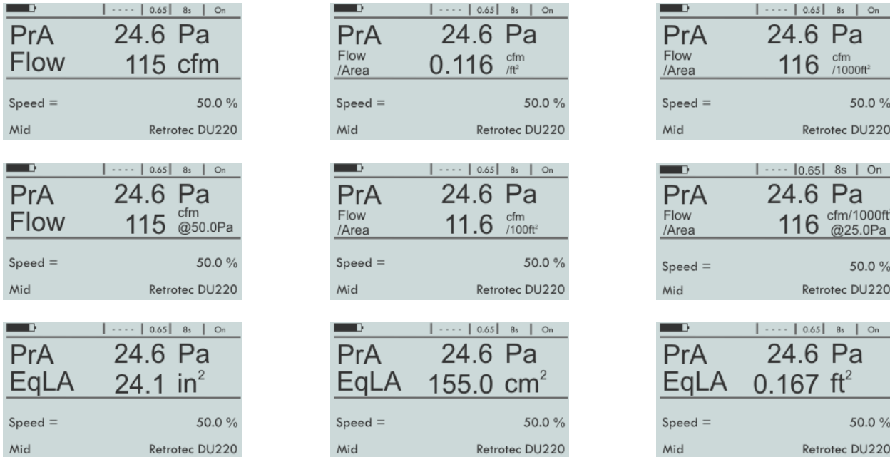
Figure 34. Some of the most common results that can be read directly off the DM-2.
