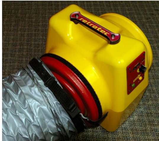
Figure 16. Install Flex Duct over the fan inlet for depressurization.
