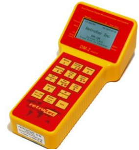
Figure 9. DM-2 digital gauge.
