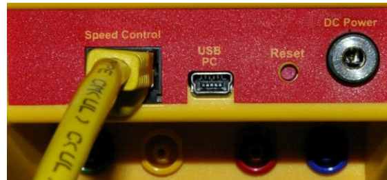
Figure 14. Electrical connections on the back of the gauge include Control Cable that goes to the DM-2 (shown connected), USB cable for a PC, reset switch and DC power connection.
