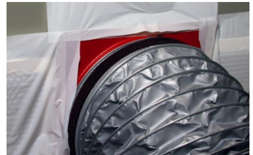
Figure 24. Flex Duct connected to the Flange.
