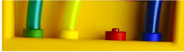
Figure 13. Pressure ports on the back of the gauge are color-coded to match the tubing.
