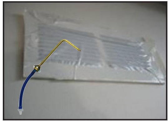
Figure 25. A Static Pressure Probe attached to a pressure tube allows the measurement of pressure without flow interference (e.g. inside a supply register)
