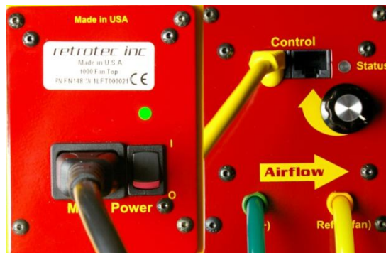
Figure 15. Model 200 Fan Top with power cord, color-coded tubing connections (green and yellow) and Control Cable.
