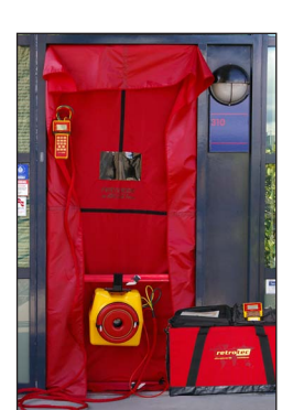
US200 Door Panel for tight enclosures. #AL214
