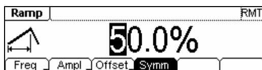
Figure 2-13 Ramp Signal Parameter Setting Interface
