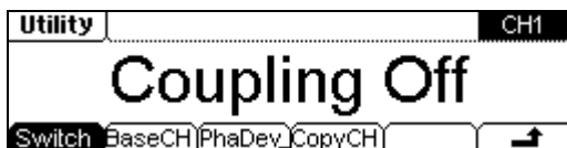
Figure 2-60 Channel Coupling Setting Interface
