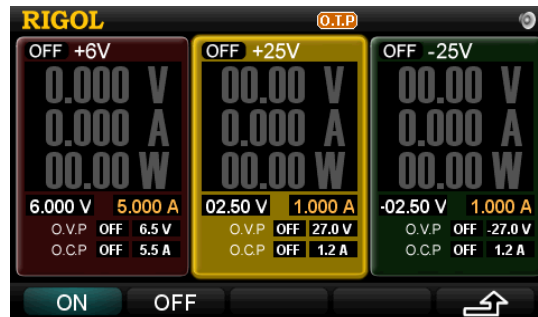
Figure 2-28 Over-temperature Protection Settings
