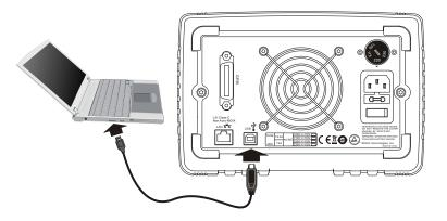
After successful connection, turn on the instrument, a dialog will guide you to install the driver of "USB Test and Measurement Device (Agilent)" on the PC. See the figure below:
