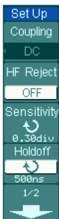
Figure 2-55 Table 2-34 The Trigger Set Up menu (Page 1/2 Settings for Edge, Pulse and Pattern Triggers)
