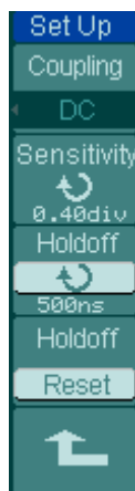
Figure 2-52 Table 2-32 The Trigger Set Up menu (Settings for trigger coupling, trigger sensitivity and holdoff)
