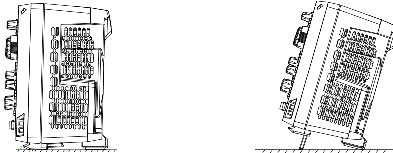
Figure 3 To Adjust the Supporting Legs
