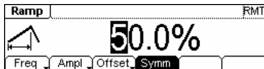
Figure 2-13 Ramp Signal Parameter Setting Interface
