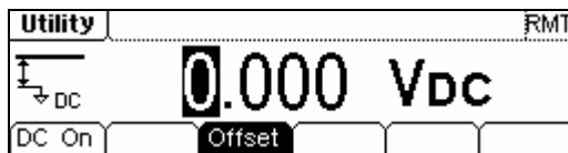
Figure 2-76 The DC Setting Interface
