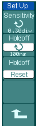
Figure 2-63 Table 2-39 (Settings for sensitivity and holdoff)
