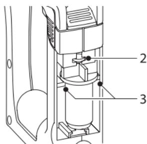
Ensure that the pump plunger (2) and pump body (3) are situated in the corresponding guides when inserting the sample pump.
