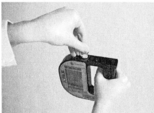
Fig. 11-4 Opening the battery cover
