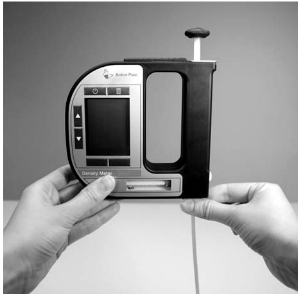
Fig. 7-1 Connecting the filling tube
