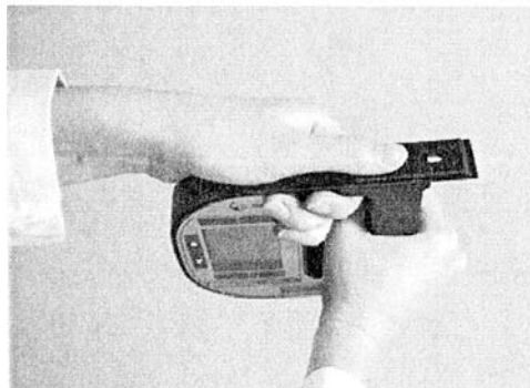
Fig. 11-3 Removing the pump lock
