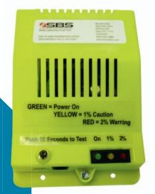
Lead-acid storage batteries emit hydrogen while gassing during charge. Hydrogen concentration of 4% to 75% by volume in air, is potentially explosive. The SBS hydrogen gas detector is designed to provide dissipation and warning before any concentration reaches the lower explosive limit (LEL) of 4%.
