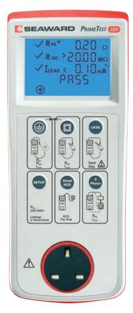
Seaward's lightweight, portable Primetest 250 PAT tester is unique in its range of safety tests. The PrimeTest 250 will perform all of the tests required by the IEE Code of Practice, including RCD trip, protective conductor current and touch current where required. The unit also includes a 250V DC insulation test suitable for testing sensitive electrical appliances and surge protected leads.
