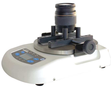
Camera Lens Zoom testing
