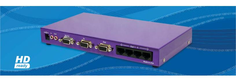
Use a single cat5 cable to broadcast high resolution SXGA, Stereo Audio, RS232 and IR to 4 stations up to 1000ft away.
