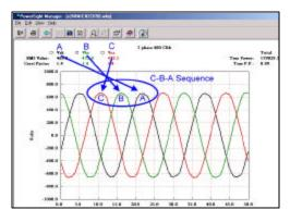
starts at a different place (for instance B-C-A is just a portion of the continuing sequence of A-B-C-A-B-C). Sometimes an order of C-B-A is correct. Some utilities deliver power in that sequence and sometimes a motor will be connected in that manner to make it spin "backwards". An order of B-A-C or A-C-B is the same as C-B-A, the reference point just starts in a different place (for instance B-A-C is a portion of the continuing sequence of C-B-A-C-B-A).
