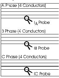
needs. However, experience shows that although the current in each conductor of the same phase is similar in size, they are typically NOT identical.
