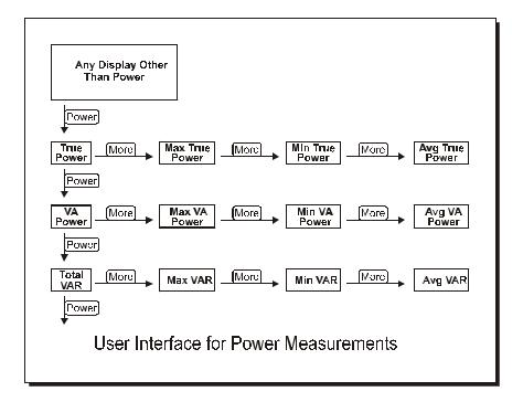
For instance, if the maximum reactive power is desired, press: [Power] (to display watts), [Power] (to display VAR), and then [More...] (to display maximum reactive power).
