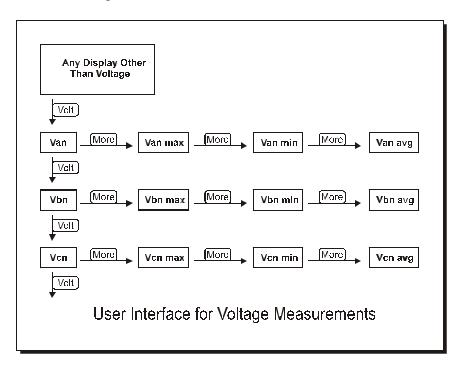
For instance, if the average voltage between Vb and Vn is desired, press: [Volt] (to display )Van, [Volt] (to display Vbn), [More...] (to display maximum Vbn), [More...] (to display minimum Vbn), and then [More...] (to display average Vbn). Note that if PowerSight is not monitoring consumption, the maximum,
