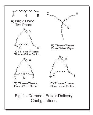
loads are encountered, Vab (240V) is used by delivering both hot voltages to the load. Neutral provides the current return path. If the load is balanced, there will be relatively little neutral current. Refer to figures  $\underline{2}$ ,  $\underline{3}$ ,  $\underline{4}$ , and  $\underline{5}$  for various ways to connect to single-phase and two-phase power service.
