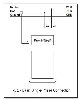
voltage now comes into PowerSight on Va and current is sensed by Ia, the power and power factor for this single-phase system will be available as phase A power and phase A power factor.
