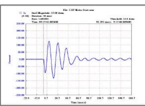
the cursor over the graph results in the voltage (or current) of that point being displayed in the heading. Whatever is seen can be zoomed-in on and can be printed.
