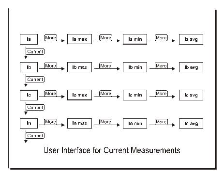
For instance, if the average current of the C Phase is desired, press: [Current] (to display Ia), [Current] (to display Ib), [Current] (to display Ic), [More...] (to display maximum Ic), [More...] (to display minimum Ic), and then [More...] (to display average Ic).
