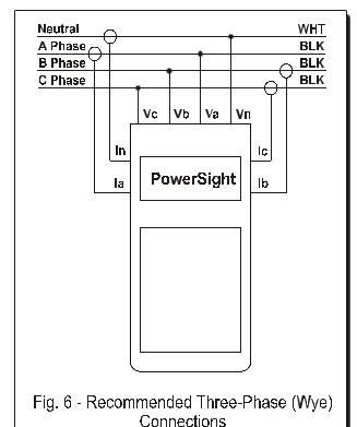
current is generally relatively small since the currents of the 3 phases largely cancel each other in the neutral leg. In a perfectly balanced system the current in neutral would be zero.
