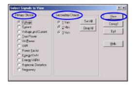
make a secondary choice of which phase or phases to view, then click on "View". Choices of measurement types that are not available in the log will be "grayed" out.
