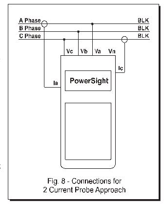
voltages of the three-phase circuit. The disadvantage of this approach is that you cannot determine the power, power factor, or VA of each individual phase and, of course, you cannot record the current of one of the active phases.
