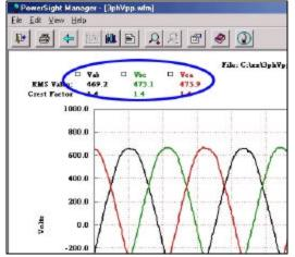
the top will be Van, Vbn, and Vcn. The first letter after the "V" is the phase that is connected to and the "n" stands for neutral. If no neutral is connected to PowerSight, this measurement is in reference to the neutral point between all the phases that are
