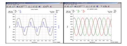
There is a wealth of features related to viewing and analyzing waveforms. Voltage and current can be viewed together and multiple phases of signals can be viewed together.
