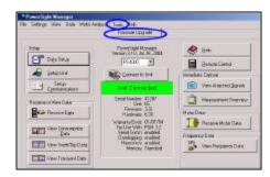
then click on Upgrade. The process will take about 2 minutes at 57.6 kbps. For detailed instructions, examine the application note UpgradingFirmware.pdf located on your installation CD.
