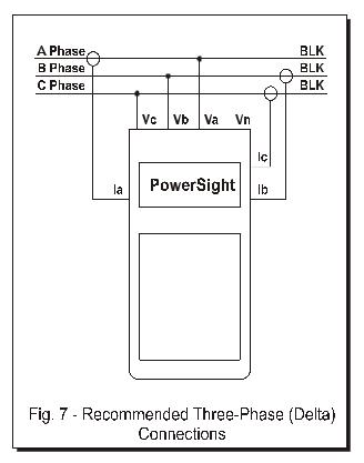
Please Note: Do not connect the Vn input to anything when measuring in phase-phase measurement mode. This may affect the accuracy of the measurements.
