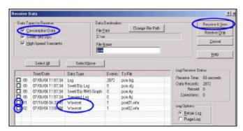
look for the "Waveset" Data Type lines. These files are the stored waveform sets stored in the PowerSight. Make sure that the box at the start of the line is checked and then click on "Receive and View" to transfer the waveform set to your computer. The default name of the file is psm01.wfm.
