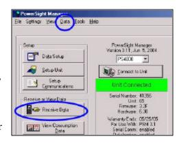
Data" button or on the "Data" dropdown button and then "Receive Data". In either case, the Receive Data menu will open and all the different types of data files in the connected PowerSight will be displayed.
