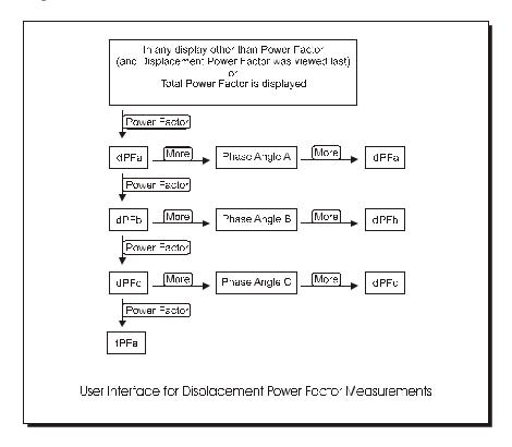
In this way, by combining the [Power Factor] and [More...] keys, there are 6 displacement power factor and phase angle measurements available.
