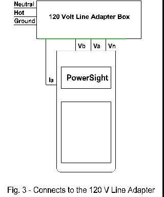
Note: Make sure that the hot and neutral wiring being measured is not reversed. If so, PowerSight and its attachments will "float" at 120 V.
