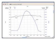
You can easily transform any waveform into either a graph of harmonic data or a view the raw data for each harmonic and K factor. To convert a waveform ("time domain" representation) into a
