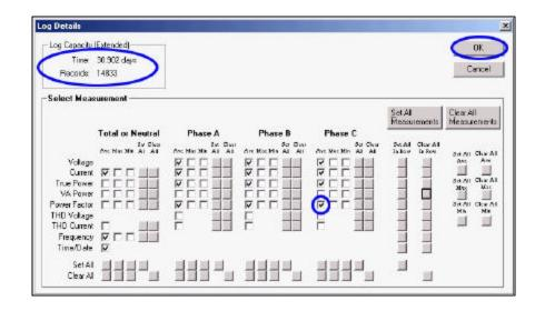
As measurement types are added or removed, the capacity of the log is affected. If fewer variables are saved, then each log record is smaller and thus more records can be stored in the log, which means that it will take that much longer to fill the log. In the example shown, there is a capacity of 14,833 records in the log which combined with the logging period of 3 minutes, will take 30.9 days to fill up.
