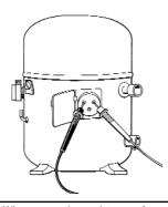
When measuring resistance of a motor, make sure the power is disconnected prior to testing. Set up meter following steps under "Measurement Procedure" on page 16, and proceed with the following:
