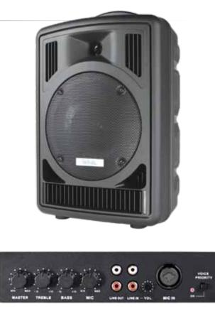
Titan AC/Battery powered portable sound system (basic unit). The Input Panel provides a Lo-z XLR Microphone Input with Volume Control, Stereo Line Input with volume control and Dual Line Output, Treble & Bass Controls, Master Volume Control. Voice Priority Button with LED.
