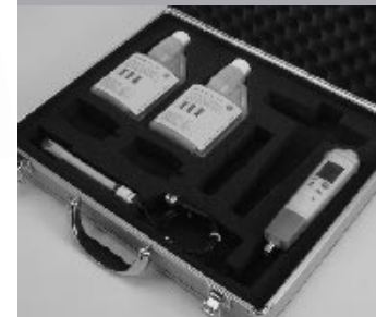
One-hand pH/°C measuring instrument, pH3 probe head with BNC interface, pH probe Type 01, storage cap with gel, calibration dosing bottles 250 ml pH 4+7, TopSafe, belt/wall holder and aluminium case
