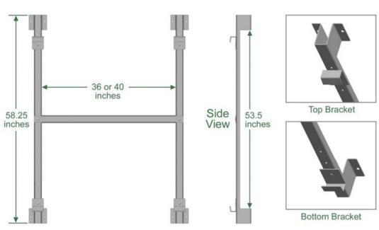
**Diversimount** employs a unique system of two uprights with a cross member and 5 lower mounting positions with variable length slots at top truly making it a "one size fits all" solution! **Diversimount** also borrows some key design elements from our flagship track mount system, **Diversitrack**. Namely our flexible clip system that holds tight to your favorite interactive white board.
