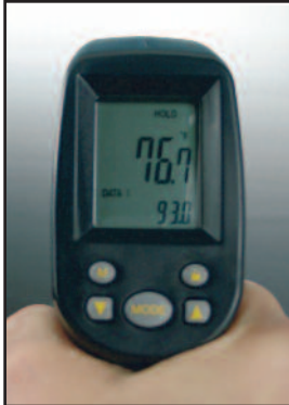
Easy to read digital display on models DHS135 and DHS215 and DHS235.
