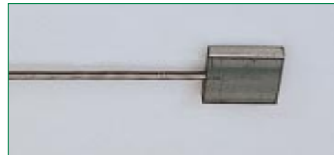
Weld-on surface probe attachment. 316 Stainless steel tab can be welded to surface to be measured. Accepts 3 or 4.5 mm (0.118" or 0.177") shank diameter probes.
