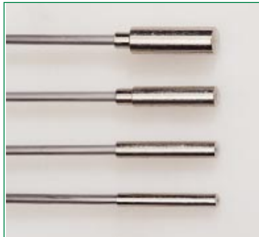
Nickle-plated brass crimp-on probe tip adapters for fitting existing mounting apertures of from 3 to 8mm (0.118" to 0.315") in diameter. Fits probes with 2 or 3 mm (0.079" or 0.118") shank diameter.
