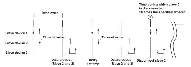
(2) Disconnect slave device 2 for a period equal to 10 times the timeout value and recover through retry at the first read cycle
