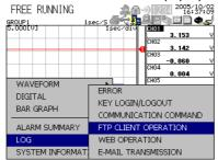
2. Use the **arrow keys** to select the desired log display, and press **SELECT**.
