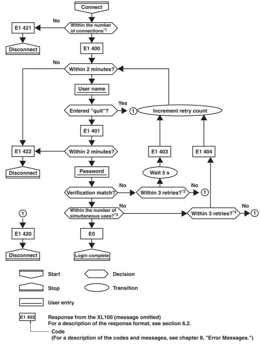
\*1 Connections cannot exceed the maximum number of connections (see section 2.1).
