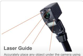
Accurately place any object under the camera using the patented laser positioning guide.
