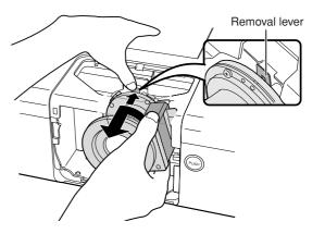
Remove the lens cap from a replacement lens.
