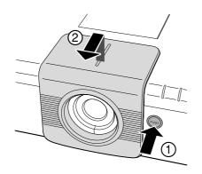
Turn the lens in the direction of the arrow while pressing the lens removal lever to pull the lens out.
