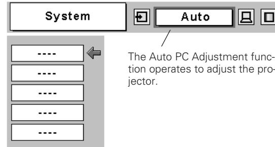
The Auto PC Adjustment function operates to adjust the projector.
