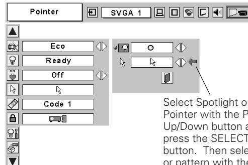
Select Spotlight or Pointer with the Point Up/Down button and press the SELECT button. Then select size or pattern with the Point Left/Right button.
