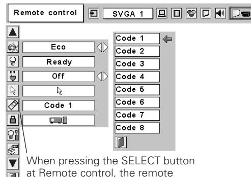
When pressing the SELECT button at Remote control, the remote control code menu appears.
