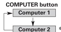
\* Computer 2 is not displayed when the COMPUTER IN 2/COMPONENT IN/MONITOR OUT terminal is used as Monitor out.
