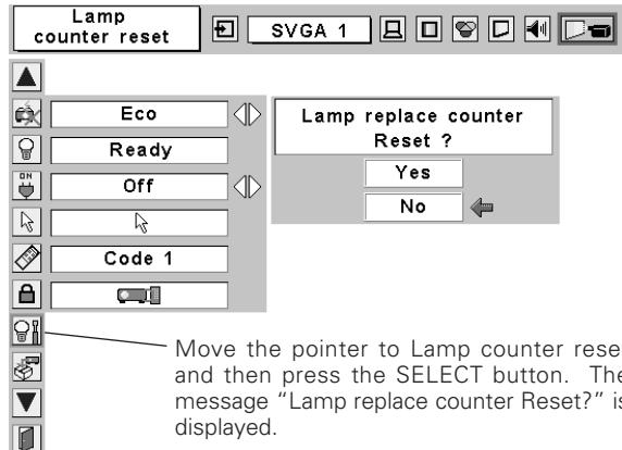
Move the pointer to Lamp counter reset and then press the SELECT button. The message "Lamp replace counter Reset?" is displayed.
