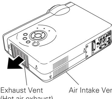
Cooling fans are provided to cool down the projector. This projector monitors internal temperature and control the running speed of the cooling fans.
