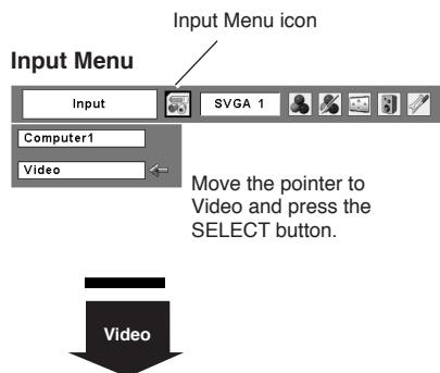
**Auto** When selecting Auto, the projector automatically detects the incoming video signal, and adjusts itself to optimize its performance. The projector selects a connection in the following order:
