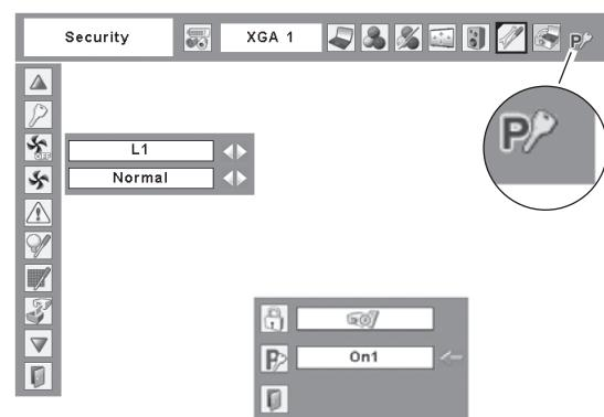
When the projector is locked with a PIN code, the PIN code lock symbol appears on the menu bar.
