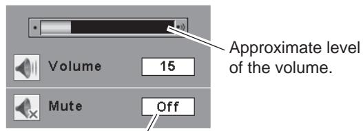
Press the MUTE button to set the Mute function On or Off. The dialog box disappears after 4 seconds.
