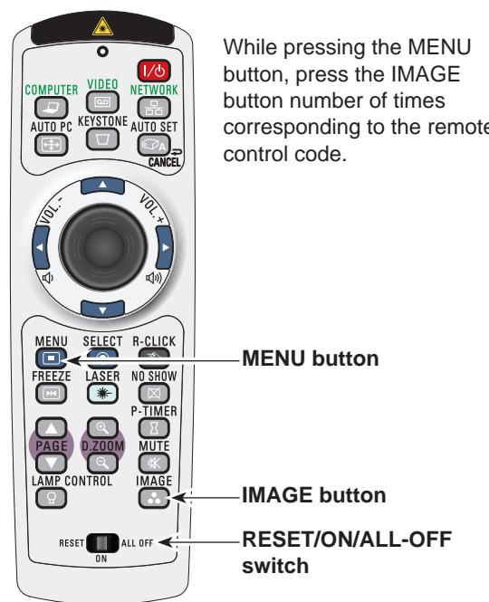
While pressing the MENU button, press the IMAGE button number of times corresponding to the remote control code.
