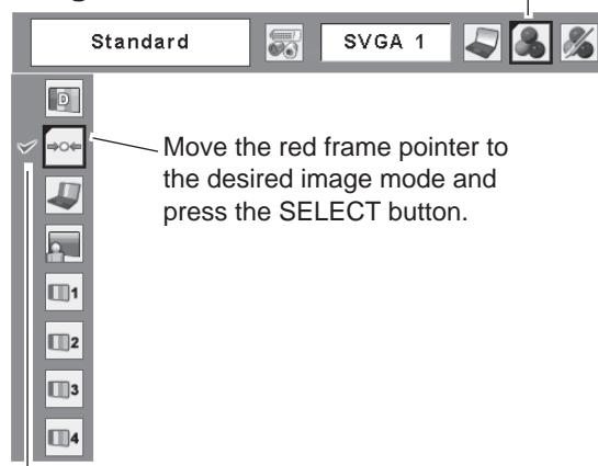
Move the red frame pointer to the desired image mode and press the SELECT button.
