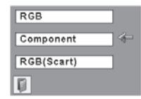
**Component** When the input source is coming from video equipment connected to the COMPUTER IN 2/COMPONENT IN terminal with a Component-VGA Cable, select Component.
