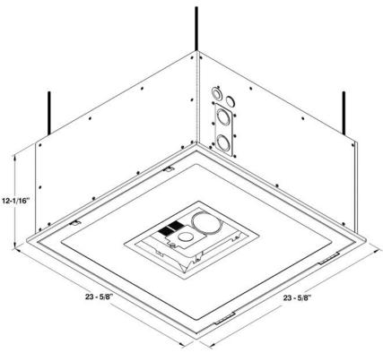
assembly placed at the very center of its adjustment range, the point that the camera lens axis (which is at a fixed 15 degrees forward tilt from vertical) exits the very bottom (main door) surface of the unit is right on the centerline of the overall front-to-back dimension of the box. This makes locating the box in the ceiling architecturally easy in relation to the lectern surface.
