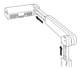
For displaying small objects or to inspect documents close-up, lower the camera arm. You can place the lens within approximately 2 inches (5 cm) of the document.
