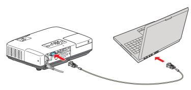
Connect the square end of the USB cable to the projector's •<--Type B (square) USB port.
