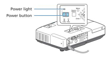
To shut down the projector, press the  $\circ$  **Power** button twice and simply unplug it. You don't have to wait for the projector to cool off.
