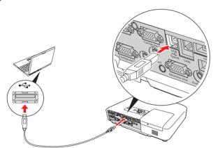
Follow the on-screen instructions to install the Epson USB Display software. (You need to install the software only the first time you connect.) Then press the **USB** button on the remote control.
