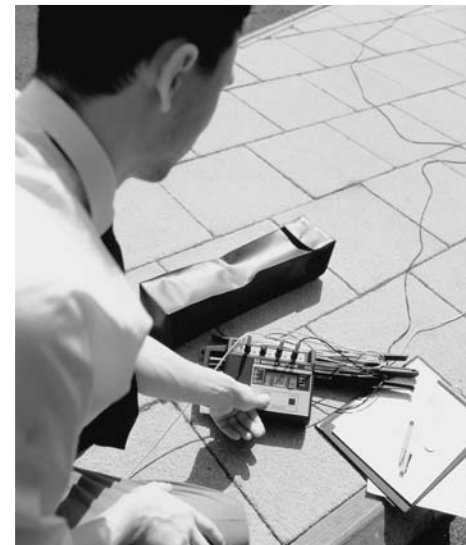
With Megger ground resistance testers' high resistance test circuits, testing can be performed on a paved surface
