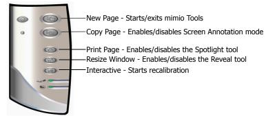
These are the default actions assigned to the mimio device buttons when working in Interactive mode. To change the actions of the buttons, see "Adjusting the Interactive Settings" on page 51.
