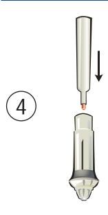
Insert the Expo dry erase marker into the Stylus Pen body that matches the Color Cap.
