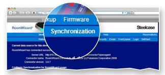
7 Under "Configure Synchronization for RoomWizard usage," select "Use external source."
