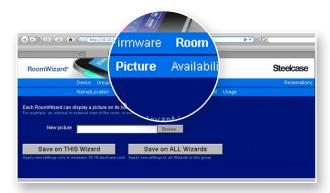
The homepage is accessed by entering a RoomWizard's IP address (not the group address) into a web browser, or by clicking the room name in a timeline. If you choose to remove the picture already inserted, you can remove it by leaving the field blank and selecting "Save on THIS Wizard."
