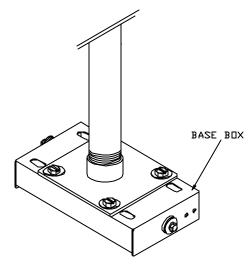
**<u>NOTE</u>:** For more adjustable suspension the PP-5 can be mated directly to our ASA-2446 suspension adapter using four (4) M10 x 25mm nut bolts and washers ( supplied ).
