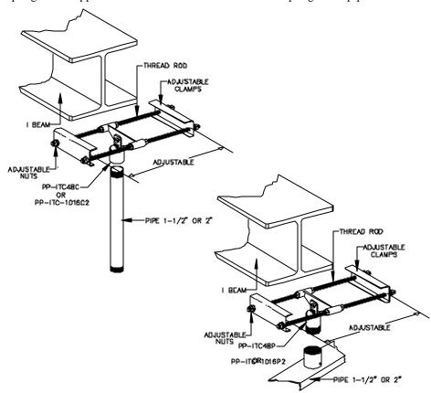
These new clamps can easily support weights up to 175 lbs. (1 ½) fittings and 350 lbs. (2") fittings properly installed by qualified personnel.
