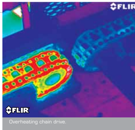
Mechanical Discover overheated bearings, linkages, and other components before they can interrupt your operations or create safety hazards.
