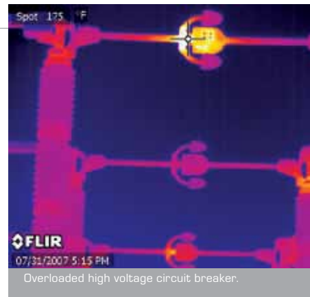
Utility Scan large areas and hundreds of connections quickly and efficiently to prevent unexpected service outages and lost revenues.
