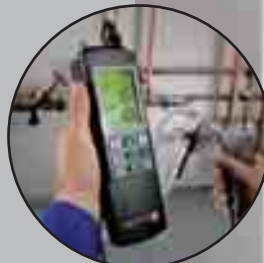
Pressure tests on waste water and drinking water pipes.
