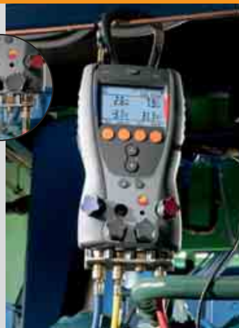
Measurements on a heat pump
