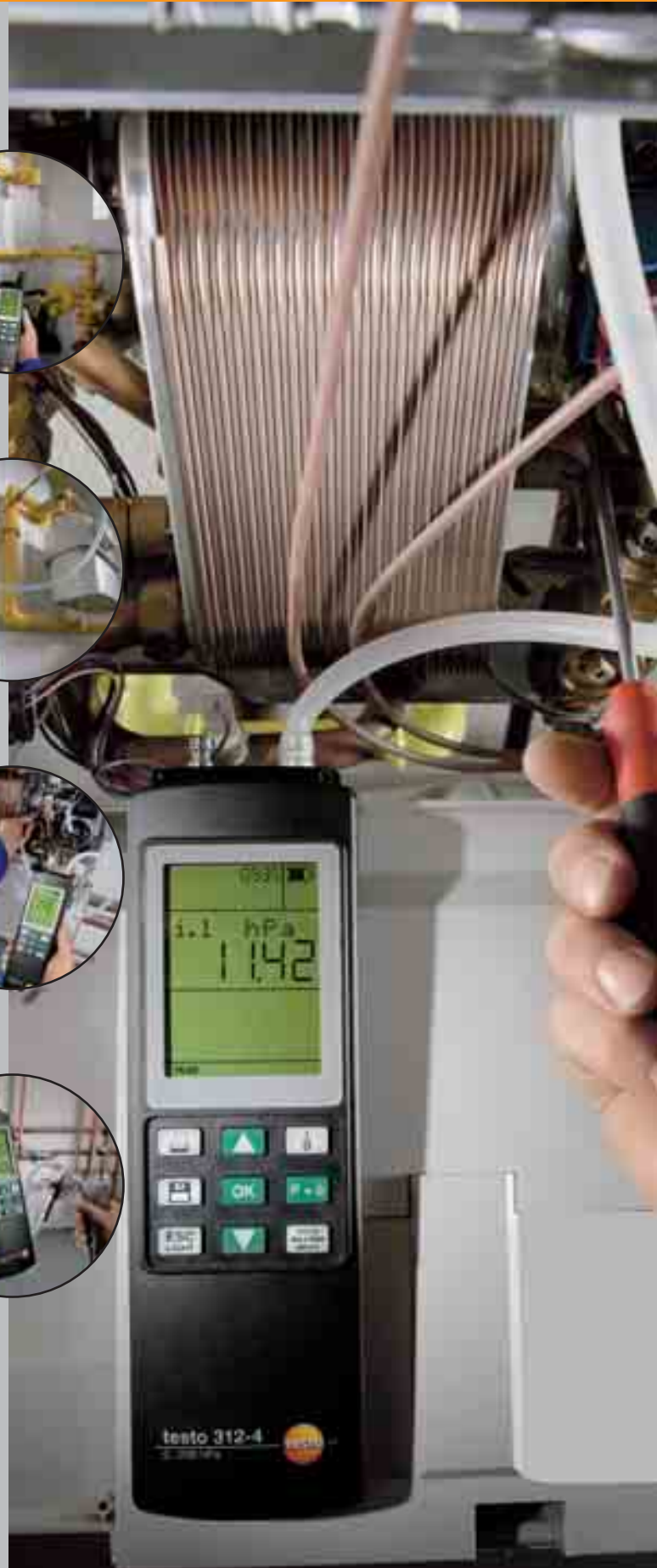
Load, gas-tightness and serviceability test by pressure drop on gas pipes as a load test for newly installed pipes
