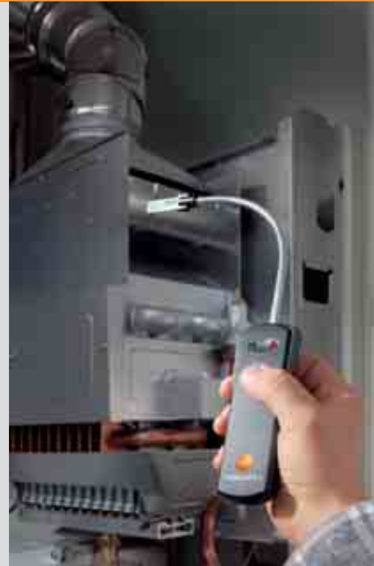
Establishes if flue gases have been drawn off completely from the burner
