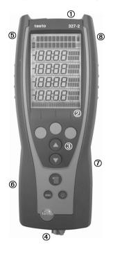
① Head: IR interface (327-2: IRDA) for connection to Testo protocol printers, ON/OFF switch (⑥), condensate outlet.
