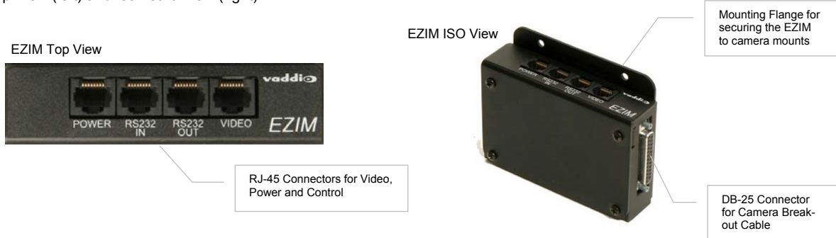
Figure 3: EZCamera Interface Module (EZIM) with four (4) RJ-45 connectors for POWER, RS-232 IN & OUT and VIDEO (HD with IR), Top View (left) and Isometric View (right)
