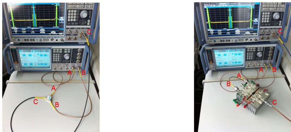
Fig. 3-1: Apparatus for calibration of the input test cables (A and B) with a resistive splitter, whose third port (C) is connected to the FSW (left). Also shown with DUT connected, post-calibration (right).
