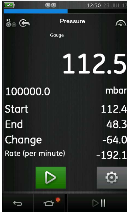
Figure 3-9 Leak Test Example
