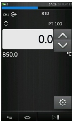
Figure 2-23 PT100 RTD Source CH1 4-Wire (Range -200 to 850 °C)
