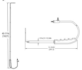
The Model 166T Telescoping Pitot Tube is a convenient adjustable length instrument for sensing air flow in a wide range of duct sizes, extending your reach to 36 inches (91 cm). It is ideal for almost any air velocity measurement where permanent mounting is not required. Because of the very small sensing holes on the tip, flow must be reasonably clean and free from particulates which could cause blockage.
