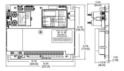
The Series DCT1000 Dust Controller Timer Controller simplifies on-demand cleaning requirements by eliminating the need for external devices such as pressure switches, relays, and timers. The modular design allows for use as a continuous cleaning control or on-demand cleaning control using the optional plug-in pressure module. The DCT1000 is the same size for 6, 10, and 22 channels, allowing one board size to be the standard on one enclosure.
