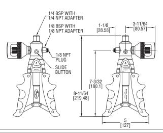
The **SERIES PCHP** Pneumatic Calibration Hand Pump sources pressure and vacuum to check calibration of gages, switches, transmitters, and recorders. The contoured cushion handles provide extra comfort while preventing the pump from sliding.
